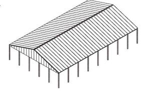
Roof Only AGRICULTURAL EXEMPT Kit contains: Galvanized Roof. Based on 25# Snow load.
